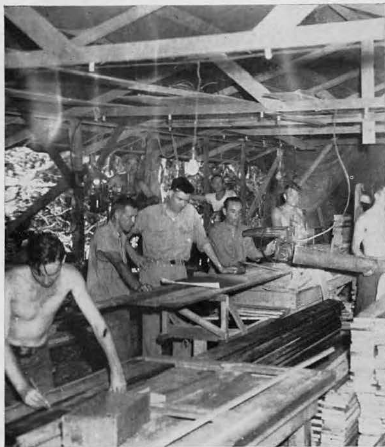
CARPENTER SHOP. Chief Carpenter's Mate "Bob" Parrott and Carpenter Karl Jehannossen (left center) study detailed blueprint at an improvised table while machine-handy assistants turn out all types of furniture from native lumber for the 87th and other units.
