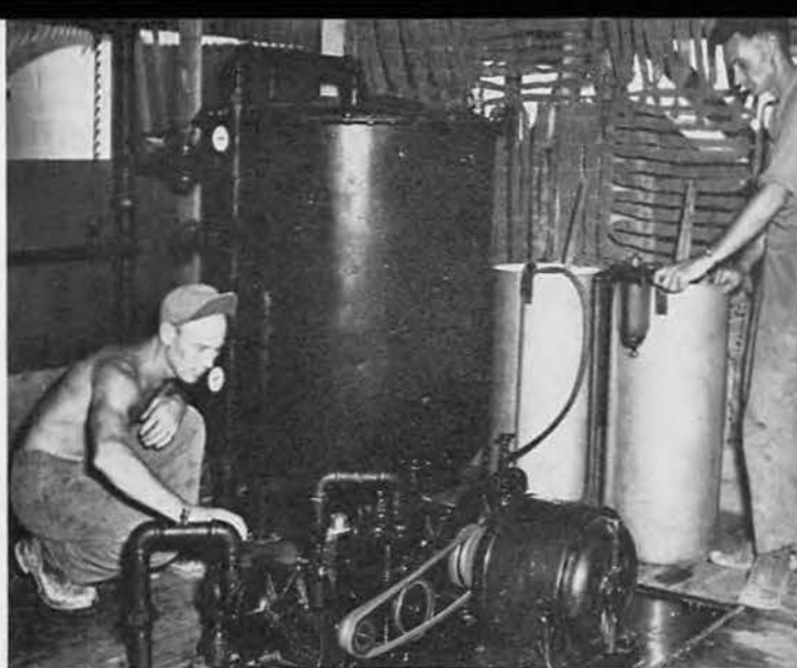
WATER POINT. Combining utility with compactness, this purifying unit and filter were built from various odds and ends and powered by a captured Jap motor. Bob Scanlon (left) and Chief Hubert Rieck adjust the unit, which handles 50 gallons per minute.
