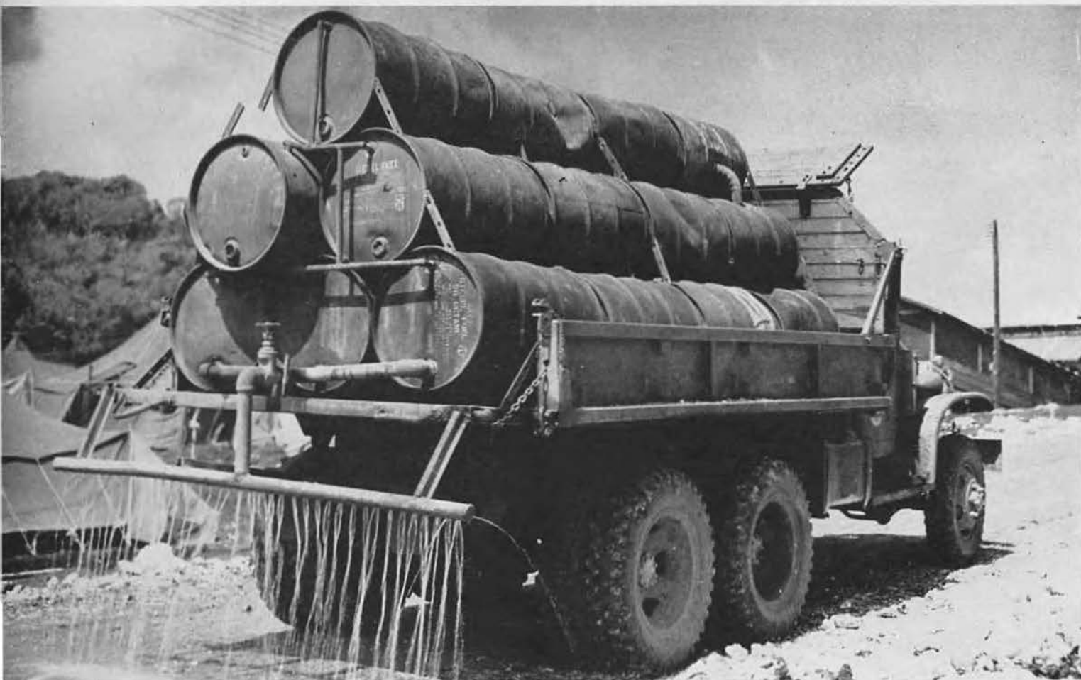
CAN DO—AGAIN! The embarrassing shortage of fresh water was in sharp contrast to the limitless supply of salt water. This ingenious contraption was "invented" by some of the more progressive element, using empty fuel drums, fashioned together by pipe. It was another illustration of what
